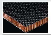
Carbon fibre material is ideal for industries that require components with high strength and rigidity without increasing weight. In other words, these products need to be really strong and sturdy but also really light. The aerospace industry revolves around aerodynamics, which is why carbon fibre is utilised to increase the quality of aerospace components without increasing the weight.
