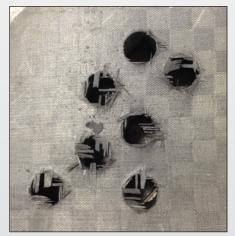
Holes drilled with CVD insert
