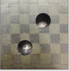
Holes drilled with Allied's T-A® PCD insert
