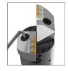
Step 5: Tighten the mounting screws on the cartridge to 15-19 Nm (11-14 ft-lbf).
